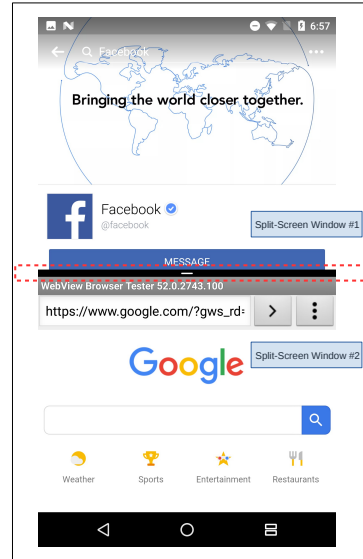
Fig. 1. A screenshot of split-screen execution in Android Nougat, where the top window runs Facebook while the bottom window simultaneously runs a web browser. The dimensions of the split-screen can be altered by dragging the black bar separating the two windows.
